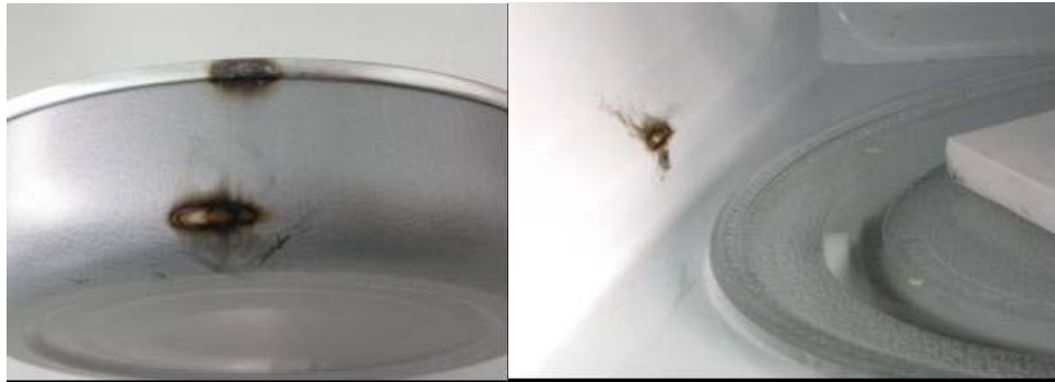
Figure 6.1: Empty \varnothing 127 container touching the oven wall in Micromaxx oven. Marks visible on container and on oven wall after several very strong sparks resulting from a number of repetitions of the experiment.
