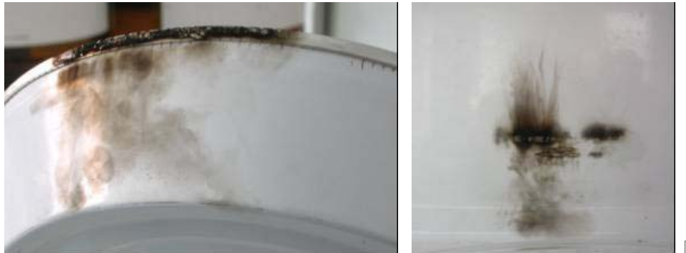
Figure 6.2: Empty \varnothing 153 container touching the oven wall in Micromaxx oven. Marks in container and on oven wall after a very strong spark. Marks on oven wall result from several experiments.
