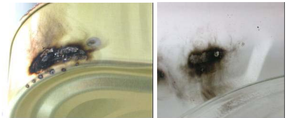
Figure 6.3: Empty \square 160x99 aluminium container touching the oven wall in Micromaxx oven. Marks in container and on oven wall after a very strong spark. Marks on oven wall result from several forced misuse experiments.
