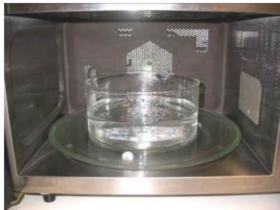
Figure 5.1: Arrangement of 1 litre tap water in a glass container for measurement of actual oven power
